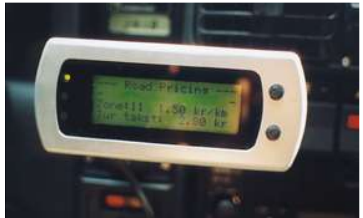
Prototype of On-Board Unit used in the Copenhagen trial
